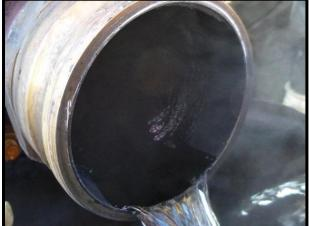
One month after the *HydroFLOW* 120i was installed - Apart for what seems like a thin magnetite layer, hard scale is not accumulating on the area that was cleaned after the first inspection. Existing scale can be flaked off with a finger and is roughly 1/8" to 1/4" thick. The customer's personnel were very surprised because typically removal of scale involves hard manual labor.
