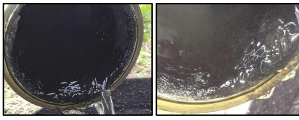
Baseline - Hard scale of roughly 1/2" along the inside of the pipe. The scale is dark because it is a mix of iron (predominantly), magnesium, calcium carbonate, silicon and other minerals.
