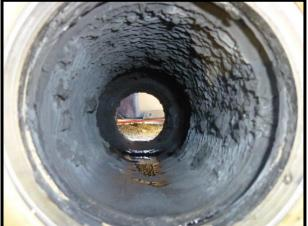
A "T" section was removed from the main line in order to inspect the inside of the pipe. It was noticed that the rate of scale removal from the bottom was much faster than the top and sides. The reason for this is because the bottom of the pipe has constant flow of water which allows scale to be removed more efficiently.
